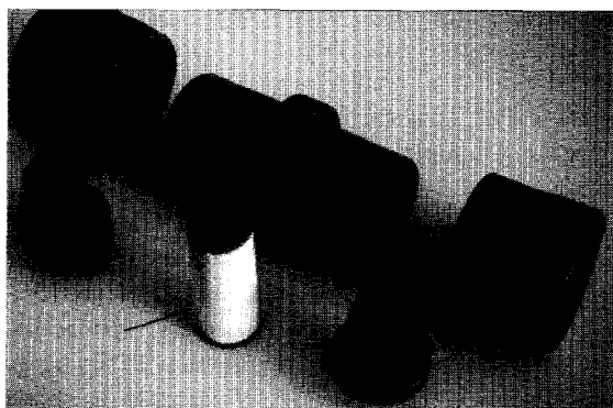
Fig. 1. Construction of the separation unit, which contains a compact porous tube (see arrow). The mobile phase or the sample is pumped from the inner side of the cylinder, flows through the wall and is collected on the other side of the unit. The separation process takes place during flow through the porous wall of the tube, as in the case of a radial column.
